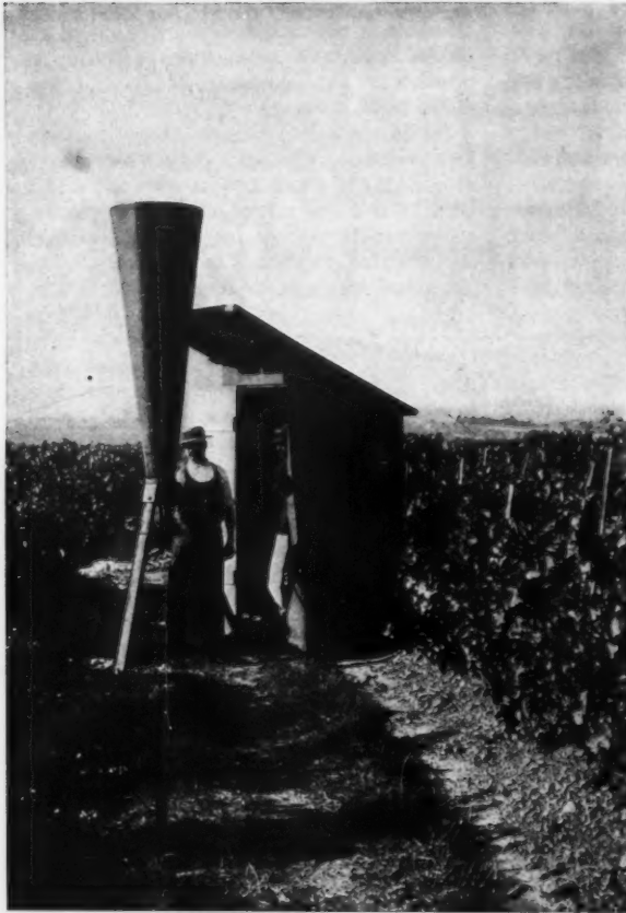
THE CANNON AND ARTILLERYMAN'S BOX AMONG THE VINES. THE ARTILLERYMAN IS IN THE ACT OF PUTTING CARTRIDGE IN THE BREECH OF THE CANNON.
