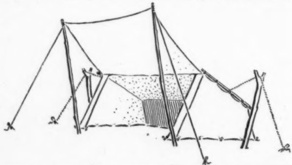
WHERE TWO TREES ARE NOT CONVENIENT, THE TENT MAY BE SUPPORTED BY FORKED STICKS, OVER WHICH THE ROPE IS PASSED, AND FASTENED DOWN BY MEANS OF A PEG. SHOWING FRONT FLAP RAISED.
