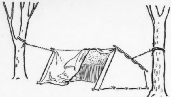
SHELTER TENT. THREE FEET HIGH, SIX FEET SIX INCHES LONG, AND FOUR FEET WIDE AT BASE.
